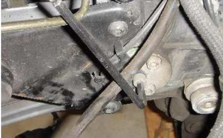
Remove the three bolts (5mm) that secure the fixed right swing arm pivot:
