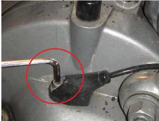
Using a narrow tool to lift the rear of it and your fingers on the front of it where the wire exits rock it back and forth while pulling up to remove it:
