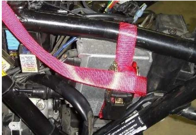
Remove the two bolts that mount the rear of the starter to the transmission:
