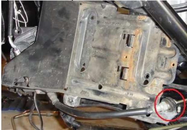
Secure the ABS control unit to the left frame rail to keep it out of the way:
