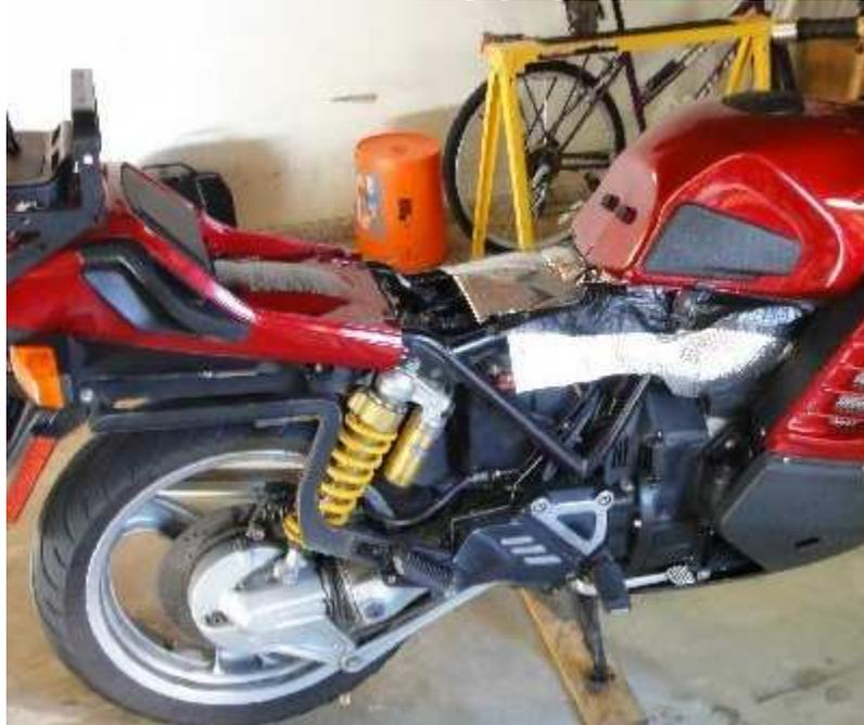
Remove the lower left side "Z" rack bolts(5mm) and the left peg plate bolts.(8mm)
