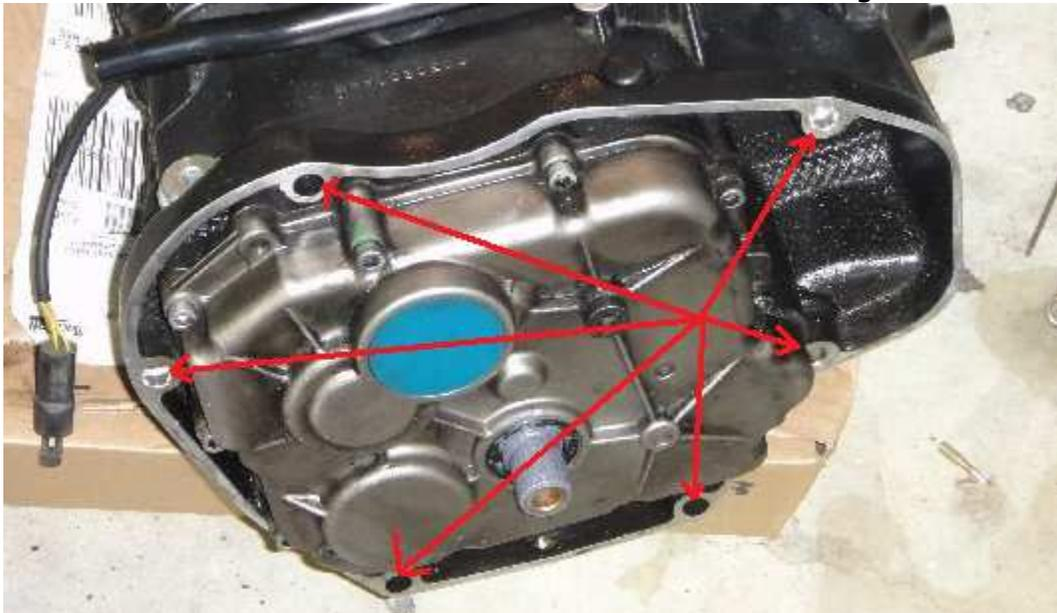
Remove the two 8mm bolts (one on each side) that mount the transmission to the frame.
