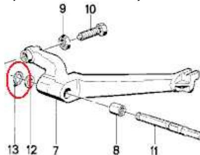
Optional: Remove the rubber boot and clutch pushrod parts. Inspect the boot to make sure it's in good shape and replace it if necessary. Pulling the clutch push rod will make it easier to get the transmission back on later after you've lubed the splines.
