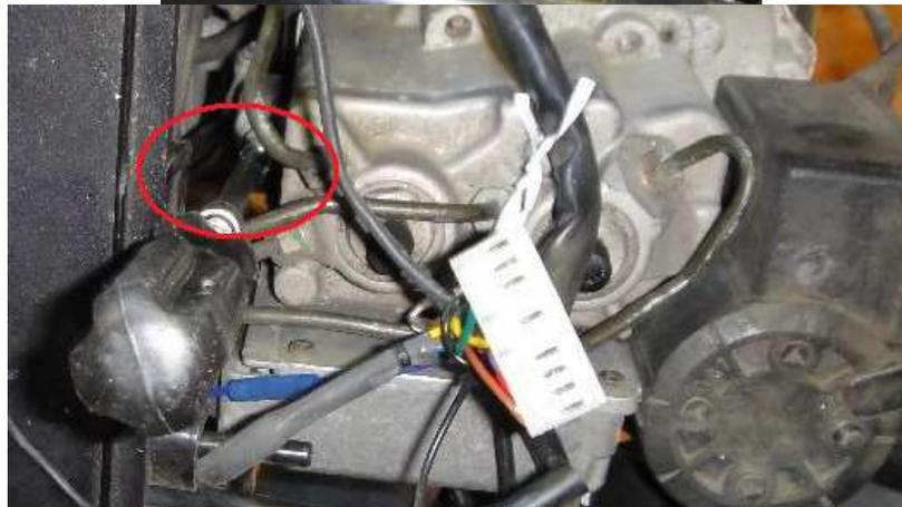
Remove the Torx bolt from the rear side of the ABS control unit bracket. I didn't have any Torx bits available so I used Vice-Grips to remove it and then replaced with a stainless steel M6x15 buttonhead Allen bolt when I put things back together.
