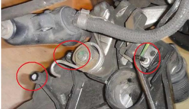
In my case my cruise control servo unit rests under the seat so I needed to disconnect the wiring harness and vacuum hose for it:
