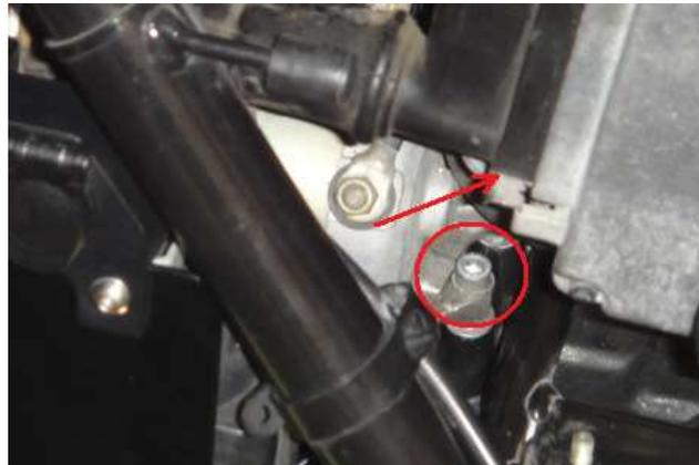
Note that you do not need to remove or disconnect the starter. Just make sure the transmission doesn't hit the starter when you slide the transmission back on.
