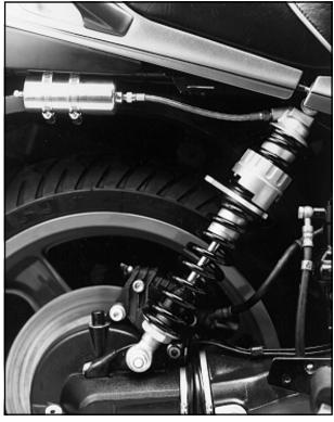
FIG. 1: TYPICAL SHOCK MOUNTING AND RESERVOIR POSITIONING FOR ALL K-SERIES BMW
