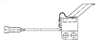
This switch can be used in place of the plunger-type switch on all K-models utilizing the **solid mount** type foot rest plate, which has an additional casting rib and mounting hole. (This switch was introduced during the 1987 production year). When installing the switch, ensure that the Switch Mounting Plate is resting against the cast rib of the footrest plate (see arrow).
