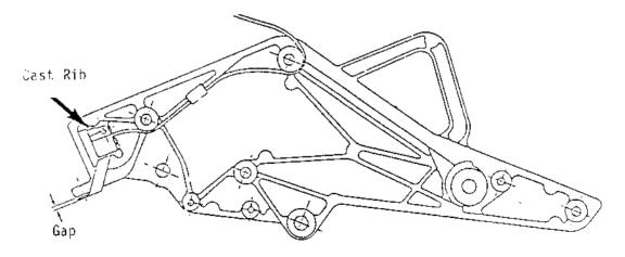
The switch is positioned correctly when there is a slight gap between the Levering Tab and the Foot Rest Plate. When the switch is correctly positioned, a click can be heard when the Foot Brake Pedal is depressed.
