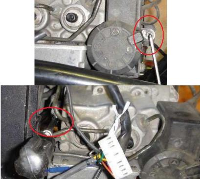
Remove the Torx bolt from the rear side of the ABS control unit bracket. I didn't have any Torx bits available so I used Vice-Grips to remove it and then replaced with a stainless steel M6x15 buttonhead Allen bolt when I put things back together.
