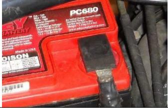
Undo the negative battery terminal first. This avoids the risk of your tool shorting to the frame when you're removing the positive terminal. Then undo the positive battery terminal.
