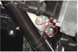
Note that you do not need to remove or disconnect the starter. Just make sure the transmission doesn't hit the starter when you slide the transmission back on. Also note that the left starter bolt grounds the coils and the right bolt holds two other ground ring terminals.
