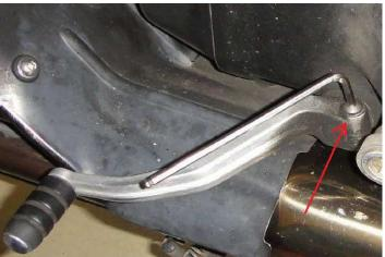
Unscrew the exhaust O2 sensor connector. (Not required on bikes in countries where they're not equipped with a catalytic converter.) Also snip the small zip tie that secures the O2 sensor wiring to the rear of the ABS control unit bracket.
