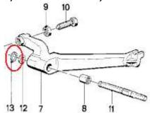
Optional: Remove the rubber boot and clutch pushrod parts. Inspect the boot to make sure it's in good shape and replace it if necessary. Pulling the clutch push rod will make it easier to get the transmission back on later after you've lubed the splines.
