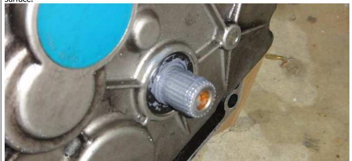
Don't worry about putting too much spline lubricant on. It will be pushed out of the collar on the clutch plate and spin off harmlessly onto the inside of the bellhousing.
