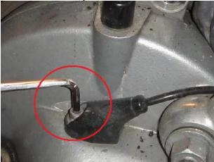
Using a narrow tool to lift the rear of it and your fingers on the front of it where the wire exits rock it back and forth while pulling up to remove it:
