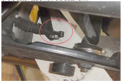
Then pull the rubber boot up through the hole in the transmission casing.
