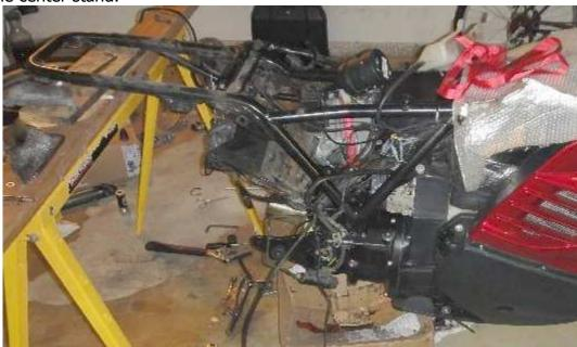
Remove the four 8mm bolts that hold the side/center stand assembly to the bottom of the transmission.
