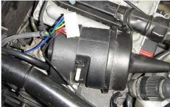
Disconnect the Motronic control unit wiring harness connector by pushing the metal tab at the rear of it back and lifting up the rear of the connector:
