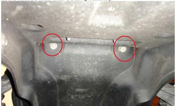
Undo the two 10mm nuts for the bracket that holds the front half of the rear fender:
