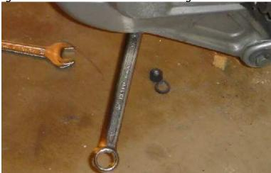
Undo the two bolts (8mm outside, Phillips machine screw inside) that hold the front half of inner rear fender to the rear half of the rear fender:
