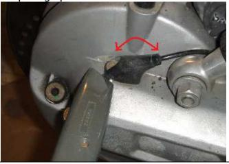
Note that there is usually some dirt gathered behind the speedometer sensor so be careful not to let any of that fall into the final drive. Once I get the speedometer sensor out I stick a finger in that hole to keep dirt from falling into it while I use the other hand to clean the dirt away:
