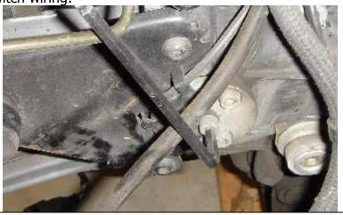
Remove the three bolts (5mm) that secure the fixed right swing arm pivot:
