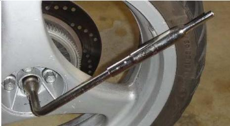
Remove the drain plug from the final drive and drain the gear oil:
