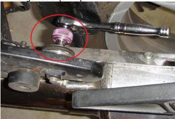
In my case the bike has a Remus exhaust so all I needed to do next was undo the exhaust clamp at the collector to remove the exhaust can. For a stock exhaust, since it's all one piece, you'll need to remove the belly pan (K1100RS only) and undo the 8 12mm nuts that attach the header flanges to the cylinder head to get the exhaust off. You might need a deep well 12mm socket for this.
