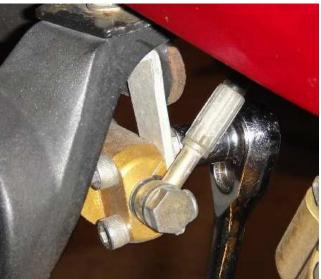
Remove the nut that holds the bottom end of the shock to the final drive:
