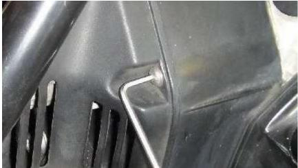
Remove the two mounting bolts (8mm) for the rear brake caliper and use some string to tie it off to the frame so it's not hanging by it's brake lines.
