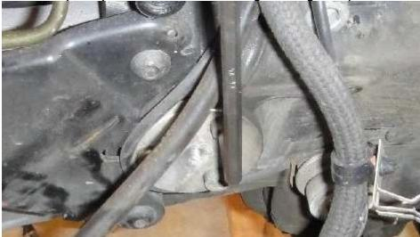
Remove the two small bolts that hold the alternator cover on:
