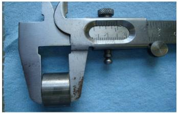
This spacer bushing is too long for use with the new slip-ring seal.
