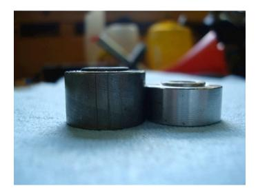
The original seal on my K75S used a spacer bushing 14mm long.
