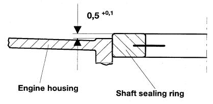
**Important:** With tool BMW No. 88 88 6 111 630 as it is currently used by the retailer organization, the shaft sealing ring is driven 0.4 <sup>+ 0.1</sup> mm below the housing edge; **therefore it must no longer be used in the present form**.
